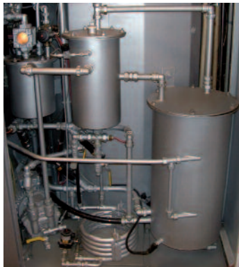
Avoids creation of odour: the multistep water separator
